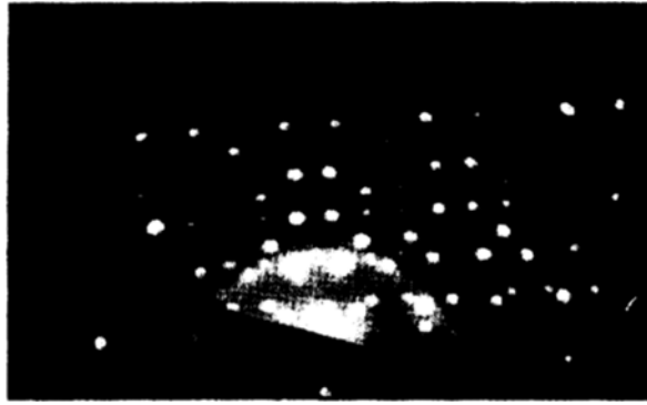
Fig. 1. Typical electron-diffraction pattern for the texture of carbon of diamond modification in the initial stage of film growth.
