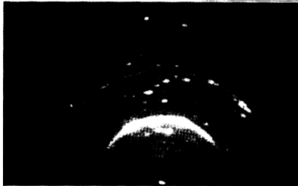
Fig. 2. Typical electron-diffraction pattern of a diamond-like film in a later stage of deposition after filling of the silicon surface with carbon.
